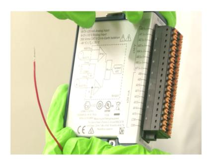
So, the first channel, so here if you see there is different number of channels starting from 0 to 7. So, total it has 8 channels for analog acquisition which can measure up to plus or minus 10 volts. So, it has both positive terminal and negative terminal. What it does is that it can measure a differential input, some cases where when you are using a quarter bridge or when you are using a half bridge or a full bridge, whatever the voltage
