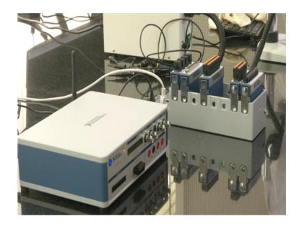
I will connect to the dc power supply. And if I vary the signals from the dc power supply, we can observe the signals being generated being acquired using this C-DAC in our monitor. So, signals can be generated using PC from the virtual bench, and the same signals can be acquired using another compact DAC, and can be acquired into this data acquisition device to the PC using this data acquisition device. And even that we can visualize.
