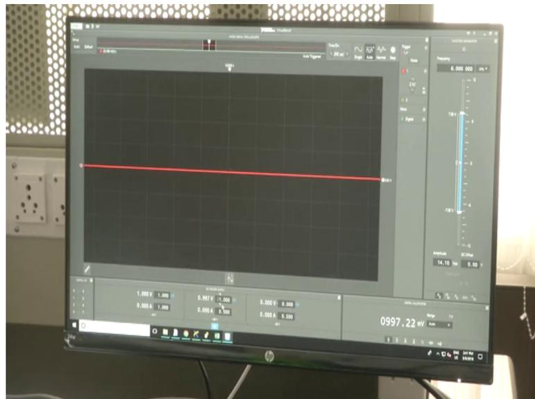
So, here this is plus 25 volts, if I increase it 1 volt 997 millivolts right. So, not only that if I want to make use of the same device to measure a resistance or to measure at to do a connectivity testing, so unfortunately I do not have a speaker connected to this, so I cannot hear it. But, there you can see the Ohms very smaller Ohms, which means that these two are shorted. So, this is the way, where you can use both a single unit as a power supply as well as a digital multimeter too.
