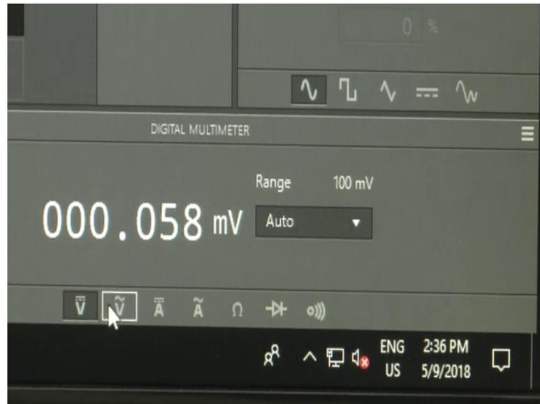
You can observe even measure DC voltage, it is a similar to that of your normal multimeter, AC voltage, DC current, AC current, resistance measurement, diode checking, connectivity checking. So, everything can be done with a single unit. Now, we will see, how we are going to use this device, and how do we measure using this particular software.
