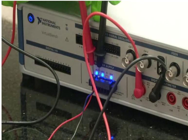
So, since I enabled, here I can observe the switching on off DC power unit the blue colour LEDs. Now, since it is connected in a voltage mode, if I measure across ground and 6 volts, so this is a variable DC power. So, here I have to go to DC voltage, so the applied voltage is 2 volts, the measured is also 2.0004 volts, see the precision of the unit.
