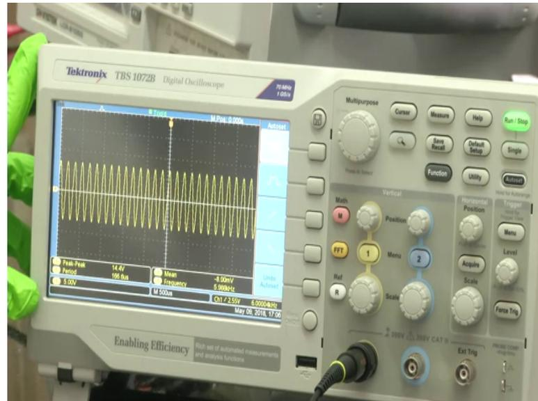
So, now what I did like, I am taking a function generator probe using virtual instrument, whatever being generated using a software or whatever being generated using this virtual instrument, we will be measuring it using the Tektronix oscilloscope. So, now in order to measure that, I will be connecting the positive terminals of both, this supply the CRO first channel input to the function generator positive input, and the both grounds, I shorted.
