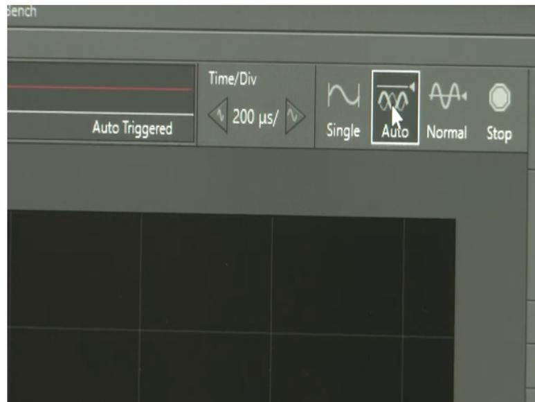
So, similar to your normal oscilloscope, you have different functionalities even here like auto setup, and changing your timescale different time scales, you can change it right. And if I want to have a single signal, you can get a single signal, auto signal, normal, and even digital so everything.
