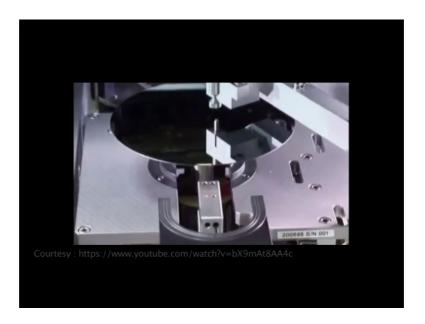
The big advantage over steppers is the exposure of the entire wafer in one step. Thus a throughput of more than 100 wafers per hour can be achieved with an overlay accuracy in the submicron range.
