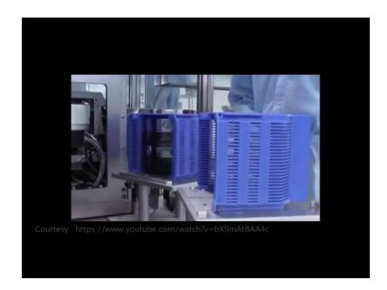
Now, I load the carrier that is all there is to it and the MA 200 compact is ready for operation. The processes of the MA 200 compact can be controlled via touchscreen.
