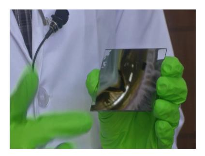
Now, what we are going to etch is, that pattern that we are going to etch is on this glass wafer ok. I am not sure whether you will be able to see the pattern, but it will be visible once the etching process completes. Now, let me quickly describe you the process flow of this. This is a 3 inch square glass wafer glass slide, where we have patterned a micro heater using nickel.
