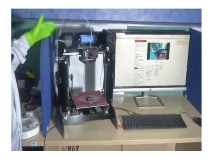
So, this is the 3D printer machine here in our lab. This here connected the thin wire if you can see is the PLA. PLA is the material which is used for 3D printing. There are really huge options regarding the choice of material for your 3D printed device and more into details will be taken to you by professor Hardik. And this is the black wire and they are available in different color combination, here the one which is right beside is the one in white.
