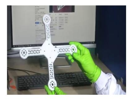
For example, the one in my hand is a 3D printed object. Now this is one part of a drone. So, as you can see the 4 hands here the structures which are here does not really go into they do not integrate any other system into this, but just that you could either have filling structure hole filling like this the entire material can be filled or you could even have structures like this in order to save material.
