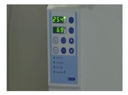
Now, this is the degree Celsius. Yeah. So, this is the degree Celsius for temperature setting, this button helps us to set the optimal temperature and it says that 37 degree Celsius is the optimal temperature for the culture growth. So, it is set at 37 degree Celsius. So, it takes time to ramp up, this is the current temperature and once we set it to 37 it takes time to ramp up the temperature and then what is the amount of CO 2?
