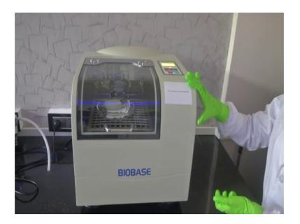
So, now that you seen how an incubator becomes an important part in laboratory for cell and tissue culture growth. Let me show you another device which is a new device in the laboratory we have not fix it yet, but this is the shaker incubator.
