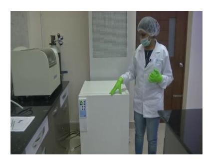
Here we have the incubator. The incubator provides the right temperature, humidity, CO 2 levels which are required for optimal culturing of cells and tissues. So, let us see: what are the different options that the incubator provides us.
