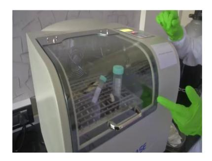
This ensures uniform mixture; the entire nutrients would be sufficiently distributed to the entire sample or the culture growth the amount of quantity that you had taken to study. So, this is the advantage what the shaker incubator can provide rather than the conventional incubator what we have already seen. Also when you want to have an incubator, look for features where you could look for programmability like increasing the temperature or setting the RPM.
