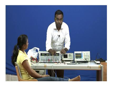
So, when we see we have already connected; we have already connected to the person. So, one we have connected to the right arm other one we have connected to the left arm. So, it has a stickiness inside as well as silica gel too. So, here at the back side we can see. the silica gel is to just to remove the impedance to decrease the impedance value and this is the at right leg position. So, this access our reference right. Now, we will take ECG connectors some using some ECG connectors.
