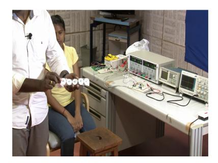
So, these are our ECG patch electrodes if you see that right. So, this is ECG patch electrodes will have a metal contact on top of it and these are not reusable; use and throw. Once we use it, we have to throw it out; disposable ECG electrodes. So, we will be placing one at right arm; one at left arm; other one at right leg because the references are right leg.
