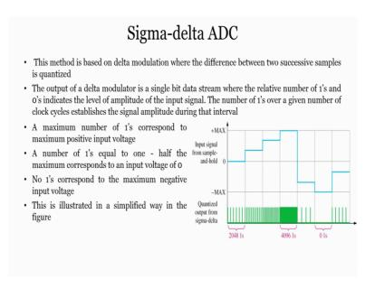
Now the final 1 would be sigma delta ADC. So, what is the sigma delta ADC means? This method is based on delta modulation where difference between 2 successive sample is quantized the output of delta modular very single bit stream where the relative numbers of 1s and 0s indicate the level of amplitude right.
