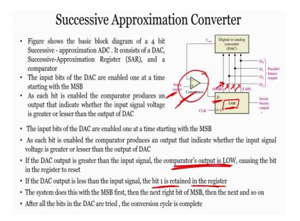
Now, if you have to understood the flash and dual slope ADC's let us see successive approximation ADC. Successive approximation ADC the block diagram is shown here when it has added digital to analog converter it has a SAR it has a digit clock and it has the serial binary output. It is connect the signal there is a digit connected is to the output of the comparator and we have a parallel binary output from D 0 to D3.
