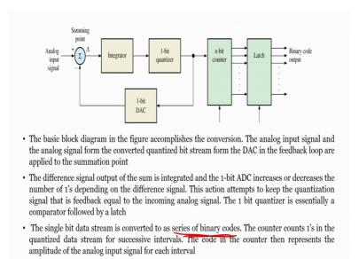
So, if you see this particular ADC right which is our sigma delta ADC and this is a block diagram when you have the integrator, a quantizer and bit counter latch. And output of the 1 bit quantizer is feed back to the 1 bit DAC which is sent to the summing point where the summing point will look at the signal sent by 1 bit ADC DAC and analog input signal and the error is fed to the integrator.
