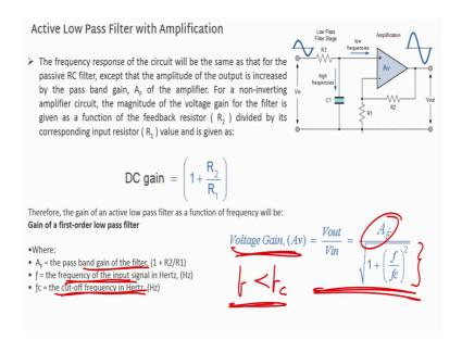
You see this one if my f is less than f C f is less than f C in this particular case right then my V out will be nothing, but A F right V out would be nothing, but A F at f equals to f C my a V out would be V out by V in would be A F by root 2 or 0.07 A F at high frequency it will be less than A F this is very simple right.
