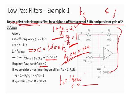
So; that means, that R f R f right should be equals to R i, we can take any value let us say 10 kilo ohms now you have value of R f R i, you have value of C you have value of R. And then you can be based on this particular values, you can design this low pass low pass filter low pass active filter right easy super easy right.
