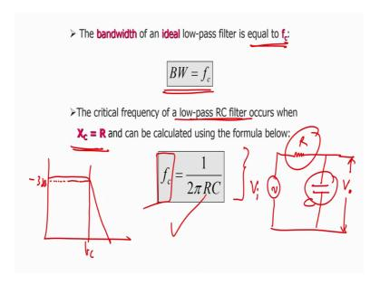
The bandwidth of an ideal low pass filter the bandwidth of an ideal low pass filter is equal to f c is equal to f c. So, bandwidth is equal to f c right the critical frequency of a low pass filter occurs when X C equals to R and can be calculated using the formula f c equals to 1 upon 2 pi RC; that means, that if I design a filter, if I design a filter then what will I have a resistor, I will have a capacitor and then I will have a output voltage V o correct CR signal right.
