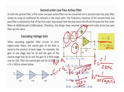
Now, let us see second order low pass active filters. So, now, if I increase one more capacitor and one more resistor one more capacitor and resistors right, it will become second order there are 2 R and 2 C gain remains same Av equals to 1 plus R 2 by R 1.
