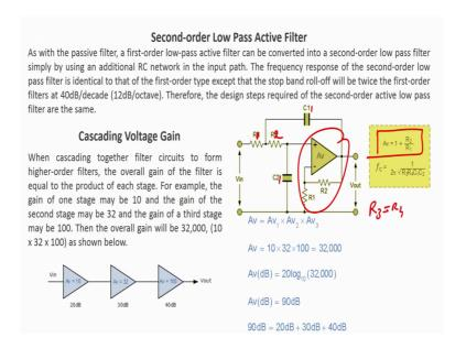
I can say C 1 C 1 2 1 that does not matter point is that there are 2 resistors, 2 capacitors and then there is of course, this inverting amplifier there is an non inverting amplifier right, there is a non-inverting amplifier the gain of non-inverting amplifier is Av equals to 1 plus R 2 by R 1 the frequency formula is 1 upon 2 pi under root of this particular 2 resistors and C 1 and C 2.
