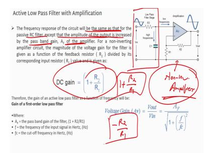
Another circuit is active low pass filter with amplification active low pass filter with amplification. So, what is low pass filter low pass filter is shown here right and here, I have connected a I have connected a non-inverting amplifier, you see here what is my circuit non inverting amplifier correct.
