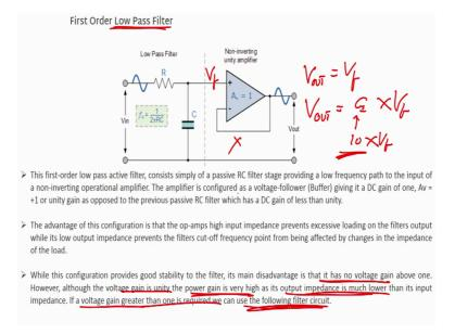
Which is a output of your filters? I will say V f output of filter, then when we see V out V out would be similar to V f, because voltage gain is it is the unity gain amplifier. So, voltage gain is 1 so; that means, that there is no actually voltage gain in the output of the operational amplifier that is the disadvantage right; however, although the voltage gain is unity the power gain is very high right.
