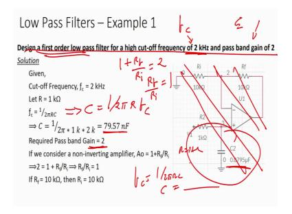
Than C would be implies C equals to 1 by C equals to 1 by 2 pi R into f c right C equals to 1 upon 2 pi R into f c. So, when you solve this when you substitute the value you know value of f c you know value of R, then you get C equals to 79.57 nano farad or this is the value right, required pass band gain is two so; that means, we have formula 1 plus R f by R i equals to 2 correct.
