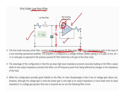
So, now if I connect a unit gain amplifier with a low pass filter which is my RC filter, it becomes my active filter. So, the first order low pass active filter consists simply a RC filter stage providing a low frequency path to the input of non-inverting operational amplifier, it is what inverting or non-inverting it is not inverting, because the signal is applied to the non inverting terminal of the operational amplifier.
