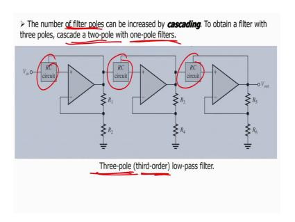
Now, number of filters now number of filters can be increased by cascading right, number of filter poles that is from 1 RC to 2 RC to 3 RC here, you can see 3 R and C right 1 RC 2 RC 3 RC right, then we see these are 3 pole or third order low pass filter.
