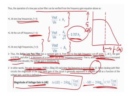
So, thus the operation of a low pass filter can be verified. So, at very low frequencies f less than f C my output would be V out by V in equals to A F right.
