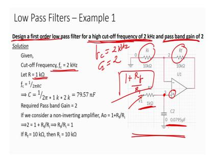
Let us see now let us see now example of low pass filter. So, you see here this circuit is given ok. So, what is the question design a low pass filter design a low pass filter for a high cut off frequency of 2 kilo hertz alright. So, we have to design a filter for the cut off frequency f C is given what 2 kilo hertz and pass band gain right pass band gain is given 2 right.
