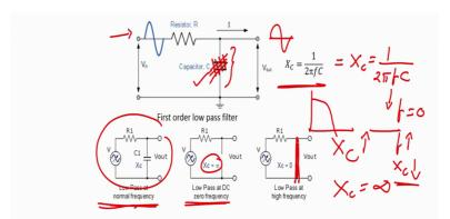
$\succ$  At low frequencies,  $X_{c}$  is very high and the capacitor circuit can be considered as open circuit. Under this condition,  $V_{o} = V_{in}$  or  $A_{V} = 1$  (unity).
