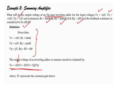
Let us quickly once again see was how what we have done with summing amplifier. Summing amplifier is nothing but an inverting amplifier corrected in a way that you have lot of input voltages more than, more than 1 voltage, now here you can see such that, you can take a summation of those input voltages can be n numbers, like this it can be until n ok, this R n in v i n, all right, n n times ok. So, point is that the formula is very easy v o
