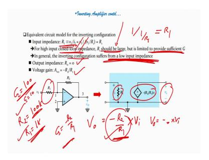
Now, if I draw equivalent circuit model of inverting configuration what will I have? I have R 1, my gain is minus R 2 by R 1 into v i I have two voltage v o input voltage v i,
