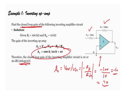
So, let us solve let us solve an example ok. Let us solve an example. So, find the closed loop gain of following inverting amplifier circuit. You have give, you are given a circuit and you are asked to find the closed loop, gain asked to find the closed loop gain ok.
