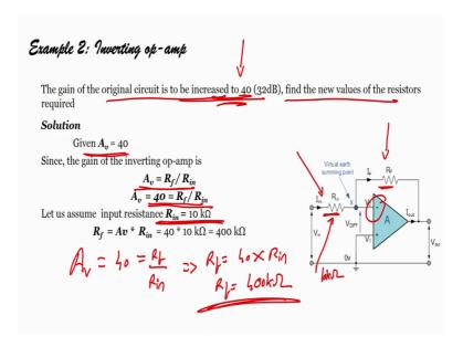
Let us see one more example; let us see one more example ok. So, the inverting amplifier the gain of the original circuit is to be increased by 40 dB ok. Find then values of resistor. See we are not given the values of resistor ok. Now, what is given? That we have to; we have to increase the gain to 40 dB or 40 or 32 dB. So, what will be the value of resistors; what will be the value of this resistors? That is the question ok.
