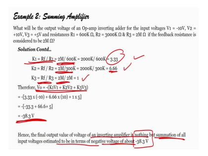
So, if I have seen the values 2 mega ohm will be a 600 kilo ohm and have 3.33 which is my R F by R 1 or K 1, same way if I substitute value for K 2 that is R F by R 2 2 mega ohm divided by 300 kilo ohm, I will have 6.66, right and then finally, for K 3 R F by R 3 2 mega ohm by 2 mega ohm is 1. So, I have now 3 values. If I substitute those values in this equation what will I have v o equals to minus 38.3, volts minus 38.3 volts.
