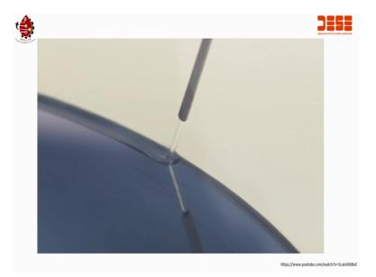
A fine needle is used and in combination with a low syringe dispense pressure. This creates a consistent stream of solvent that can be accurately directed at the edge of the substrate. The tip of the needle should be one to two millimeters from the surface of the substrate and should be angled, so that the stream of solvent flows in the direction of rotation. Laurel systems normal direction of rotation is counterclockwise.
