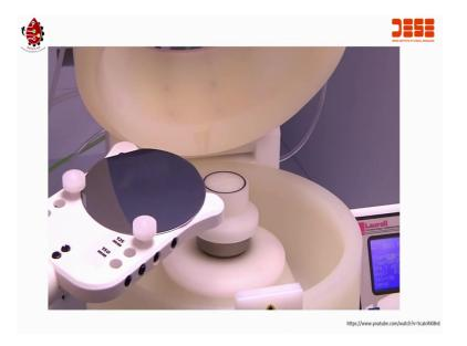
It is most important to begin with a correctly centered substrate. Here we used a laurel technologies alignment tool to guarantee consistent accurate centering. Consistent centering allows you to set up the UD-3b to accurately remove, just the edge bead without having to reset for each substrate or remove more of your coating than is absolutely necessary.
