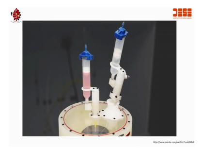
Our automatic universal dispenser is available as a fixed (Refer Time: 25:07) unit or in the off center adjustable UD-3b mount. The UD-3b is used as an additional coating dispense unit of automated edge bead removal. An edge bead is a layer of thicker material that builds up the edge of a substrate, during coating process. It can interfere with further processing steps, and is best removed as part of the coating program.
