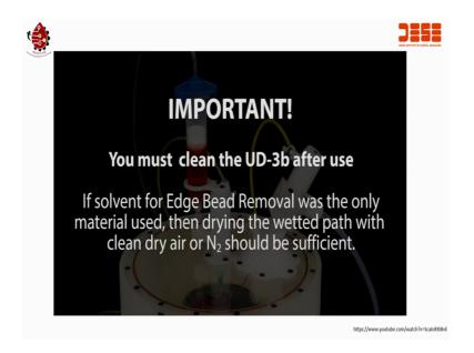
We recommend you clean the UD-3b at the end of every day. If all that has been used is solvent for edge bead removal, then drying the wetted path with clean dry air or nitrogen should be all that is necessary.
