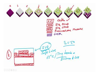
So, to do that our next step would be to spin coat to spin coat SU-8 to spin coat SU-8 on this wafer ok. If I spin coat SU-8 on this wafer, then what is my next step my next step is that I have to form the SU-8 pillars right. So, I have to first soft bake it, soft bake is done it 65 degree centigrade for 1 minute on hot plate right. This is my SU-8; then soft bake 65 degree centigrade right not 1 minute, it depends on the thickness of SU-8 right, thickness of SU-8 on a hotplate or in a oven.
