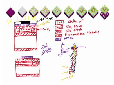
After this, what is the next step next step is, next step is we will hard bake right hard bake after hard baking, the next step is hardback is done at 120 degree centigrade for 1 minute on hot plate. After this what is a next step, next step is we will etch chrome and
