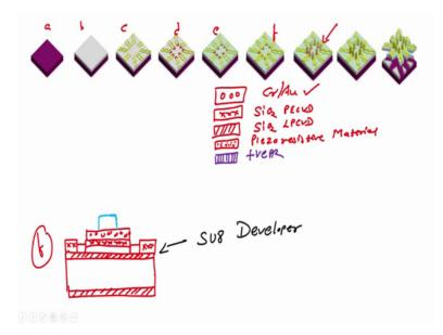
So, if I dip this wafer in a SU-8 developer, what will happen, the SU-8, we will remain only in this area right. And then I can go for further annealing at 120 or 140 degrees centigrade to make the pillar harder. This is my SU-8 patterned right to form to form SU-8 pillar right.
