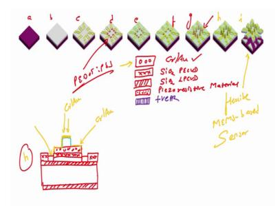
So, we will be here h right, h, what is a next step, next step is I where you had to cut the PDMS and release it to realize the to realize the flexible MEMS based sensor to realize the flexible MEMS base sensor, got it guys.
