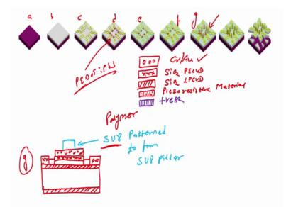
Now, in principle we will make 8 different pillars right, we will make 8 different pillars, because our sensor demands 8 pillars. There are 8 electrodes and 8 piezoresistive sensors
