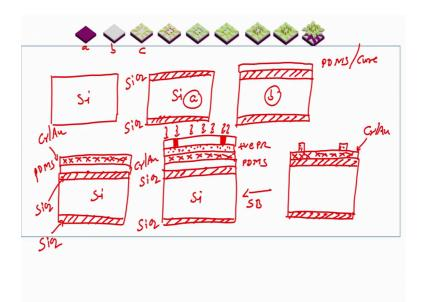
And then if I want to see how is going to work let us see, so oxidize silicon substrate. So, first is we will take a silicon wafer, next step is we will grow silicon dioxide this becomes my a, silicon dioxide. Next step is I will spin coat, I will spin coat PDMS, and cure it; spin coat, PDMS and cure it. This is my b, right.
