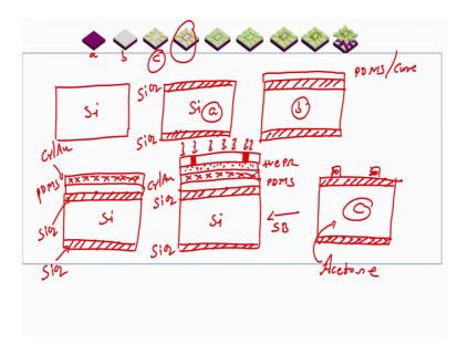
After this I will deposit or I will dip this wafer I will dip this wafer in acetone. When you dip the wafer in acetone, what will happen? My photoresist will be stripped off. When I photoresist will be stripped off what will I have? I will have contact pads, I will have the contact pads, right this is my d, this is my c c, ok. Now, what do we want? We want a piezoresistive materials, right we want a piezoresistive sensor.
