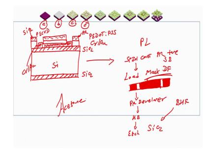
And then after that of course, after spin coating photoresist we have to do soft bake we already know that nor the mask, then do UV exposure, then you do photoresist developer right, photoresist developer, then after photoresist developer you have to do the hard bake and after hard bake you have to etch P dot PSS from the regions which are from the regions which we do not want to protect.
