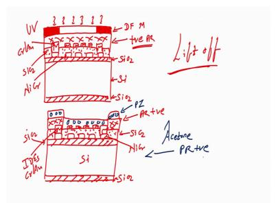
I will show you how to do lift off very interesting technique, very easy focus on the schematic that I am drawing right. I always write down even you know that what are the patterns here, what I am showing in the design is always a good practice to write down as many times as you can. So, that you remember this is using thermal oxidation over there what we have? We have a heater; over there what we have? We have a silicon
