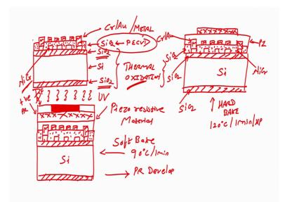
But if I have a bright filed mask; if I have a bright filed mask then I will go for a positive photoresist. So, you have to select the recipe according to the design of your mask and the ability of a photoresist right. So, here I will use positive photoresist, this is my bright filed mask easy after exposing what will happen we have to we have to develop the photoresist PR development right. If I did the wafer in photoresist which is photoresist developer then what will I have?
