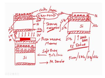
I will have a piezoresistive material over interdigitated electrodes over s i o 2 over nichrome heater and then this will look like.
