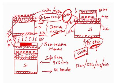
So, the point is that you know that we had a piezoresistive material all over the interdigitate electrodes and then we are protecting the piezoresistive material in this area right this much we all know, this is positive photoresist this is piezoresistive material all right this is of course, chrome gold and the main section you know. So, now, if I dip this wafer in piezoresistive material etchant, in piezoresistive etchant what will happen it will etch the piezoresistive material.
