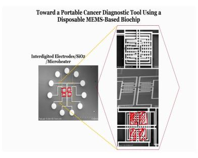
This we saw in the last module correct. Now, we will continue from this process onwards to deposit a piezoresistive material in this region, one two three and four ok. So, this is just a magnified view, this is what I want to do today and to teach you fabrication of piezoresistive sensors on the interdigitated electrodes alright.
