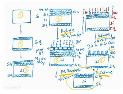
So, this everything this bio chip is made up made or fabricated on is fabricated on a silicon; silicon is a substrate. So, the first step is I take a silicon substrate, next step is to grow silicon dioxide correct because we cannot deposit a metal directly on silicon you know that. So, first is silicon, next is grow silicon dioxide. This we can grow silicon
