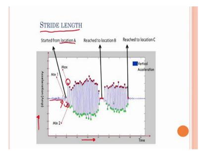
The above image shows the peaks that is the steps taken by a user for going from point A through B to C. The no peaks section at B indicates that the person stood at point B for a while and then moved onto C. The red and green points are the maxima and minima values which will be of interest to estimate stride length, that you will be witnessing in the next section.
