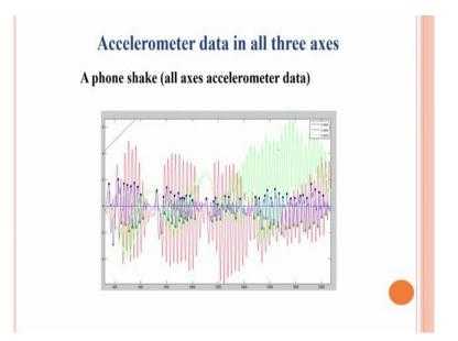
Look at this picture here, there are 3 axis results that you see here; three different colors. This is directly from a phone. The Z axis, the Y axis, and X axis are shown. This is a phone shake of all axis accelerometer data.
