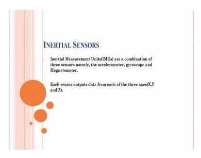
IMU sensors are a combination of 3 sensors having different principles of operation; one is an accelerometer, the other is a gyroscope and the other is a magnetometer ok.
