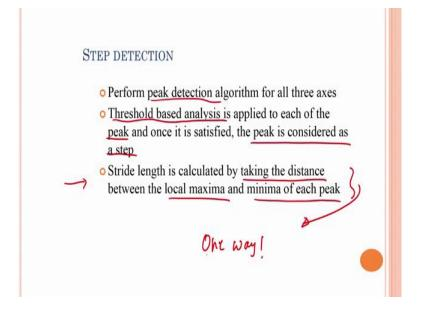
Once you perform peak detection algorithm and you apply the necessary threshold based analysis to each of the peak, then you considered a peak as a step, and stride length is calculated by taking the distance between the local maxima and minima of each peak.
