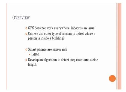
So, if you come to IMU's you will see that GPS is the usual problem. We are not looking at working with the GPS anymore and we are looking at how one can use these IMU sensors to detect people inside a building, find out where a person is inside a building and so on.
