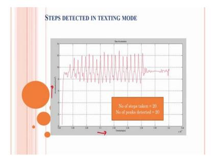
You can see that each mode has its own signatures that you will get. We also said that the unit algorithms for more recognition in any case I am just showing you some data here. These are step detected in texting mode. Again, the x axis is time; y axis is acceleration; number of steps taken is 20; number of peaks detected is also 20.
