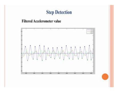
So, this is filtered accelerometer value. This is essentially the 3 axis that you have you can see that the Z axis is the most prominent. This is clearly phone is held in the hand and a person is moving forward and you can see there is a peak, there is a maximum
