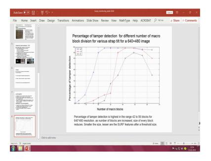
So, this is a very interesting result that we could finally, get from all of it because little bit of engineering that is associated with it. This is percentage of tamper detection for different number of macro block division, you can see that X axis is the number of macro blocks, and the Y axis is percentage of tamper detection. You can see that the result is quite intuitive the percentage of tamper detection is highest in the range 42 to 56 blocks
