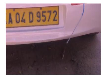
Now, let me show you a few small things. This is the car of interest that we want to measure some amount of pollution that is coming from not just the exhaust pipe which you can see here we have an exhaust pipe essentially emitting a lot of hot gases and the hot gases have to be cooled down to specified levels so that IoT sensors can essentially measure them effectively, right.
