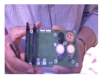
Well, what you see inside this box is essentially a bunch of sensors I mentioned to you about the different type of sensors that are there they are measuring different air pollutants. For example, the one that you see here is a semiconductor sensor we discussed this in great detail with respect to the MiCS 4514 from sensor tech which is measuring nitrogen dioxide.
