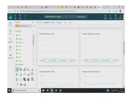
I am just juggling between exhaust and ambient just to give you a feel some sort of a comparison. Look at ammonia; ammonia in ambient is suppose to be also very low and your sensor that you require should measure anywhere quite linearly from the range of 0 to 200 ppb and you can see that is hardly any ammonia out there.
