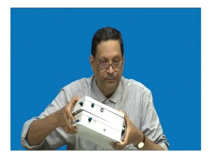
So, before you we go into the details of the graphs and other results this is what you had seen in the which were installed inside the car ok. So, in the boot space we had installed these two. As you can see one of them is for the purpose of ambient collecting ambient data the other one is with respect to the exhaust air quality, right of all the gases that we are gathering from the exhaust.
