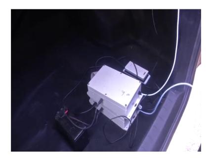
So, now I will open the boot compartment shows up and let us now zoom in to the zoom in the camera to 2 boxes which are located here and now, let us try and trace what is actually happening. This ambient air quality monitoring tube is entering this top box. You can see that the exhaust is entering a down box; is entering a box which is located below the top box; now, its clear, right?
