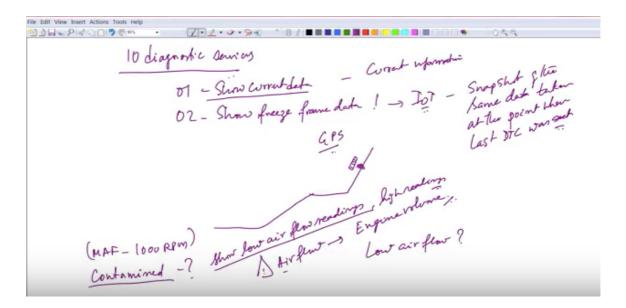
So, it is an important point you have to make a note. So, also you have to note that this low air flow. So, when you say low air flow. What does it mean? Does it mean that there is a bad sensor not necessarily? It could be the filter. The MAF could be clogged. If, you perhaps replace the air filter, the air flow may come back.
