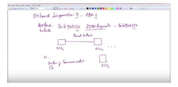
If you connect directly as shown above the ECU1 and ECU2 is a point to point link. You can have up to n ECU's as I said and each one establishing a point to point link.
