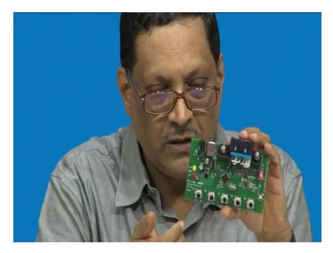
Here is an engine ECU, shown in the above picture. I drew this discussion only to tell you that this is what we want to do, we want to put this emulator simulator in action. each one of the knobs you see, there are 5 knobs. These 5 knobs correspond to different sensors as part of the engine ECU. It has essentially temperature, RPM, speed, oxygen and mass air flow.
