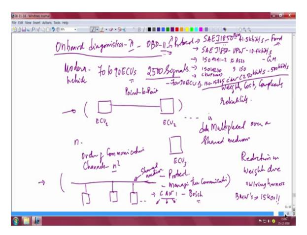
So, from 1996 onwards any vehicle that is manufactured particularly cars. There was a need for putting an on board diagnostics connector, which will give you data from all the ECU's which are there inside the vehicle.
