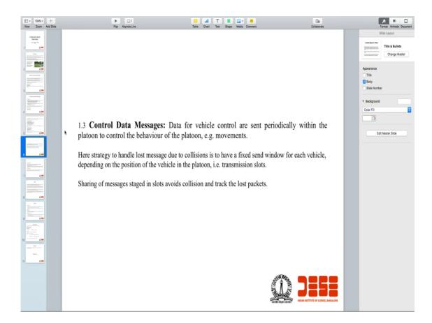
That is possible through what are known as control data messages, which are sent periodically to ensure that the platoon continues to behave, the same way the movements are same. And there are and there is a possible there is a provision to ensure, that no collision is possible between these vehicles and so on and so forth right. So, this is very important.
