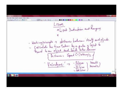
And it is based on a very simple principle quite like RADAR. If you are trying to estimate the distance between itself and some objects. You basically calculate the time taken by a pulse of light to travel to an object and back to the sensor. Very simple expression one can talk about is this distance calculation is you know the speed of light. And you know the time it takes and you know essentially if you divide by 2 assuming everything is symmetrical.
