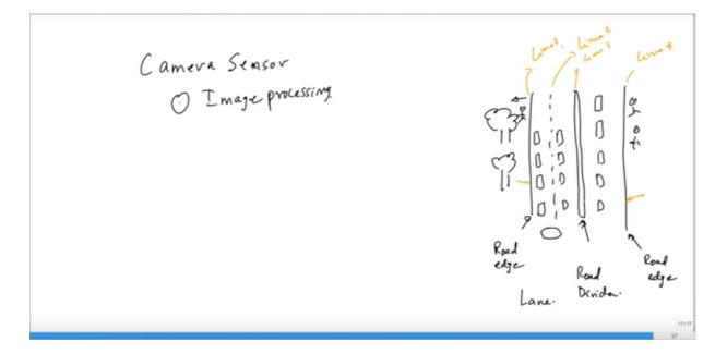
So, if you put a camera sensor on centre of the left lane and assuming that it has a good field of view. It is getting a good field of view, you are seeing all of this, which means you have to break down this image into segments and perform a segmentation of the
