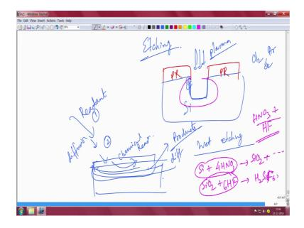
And finally, for this you know module you know this fabrication thing the one thing that is last remaining is actually etching ok, the one thing that is last remaining is etching. Etching is removal of a material for example, you have a silicon wafer and this is silicon and then you have photo resist; you have patterned photo resist.
