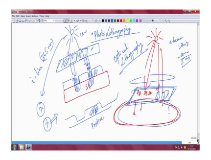
So, the next step that we should study is photolithography; photolithography is the process or the art of transferring in the pattern whatever source do in whatever you want to do the pattern is to be transferred to the wafer I told you.
