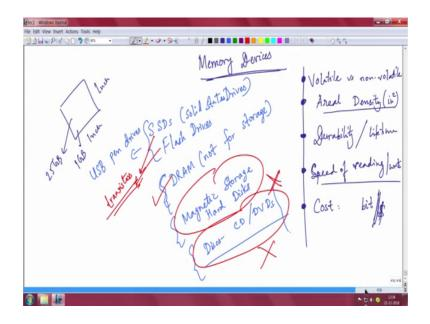
In the next we will move towards is memory; memory devices. So, what kind of memory devices used transistors and semiconductors? I am sure you probably know of many of the memory devices definitely, but you know many of the details might missing. Some of the important parameters of a memory device; what are the what are the target criteria in which you distinguish the memory devices or you classify or you rank the memory devices in terms of that performance and other things.
