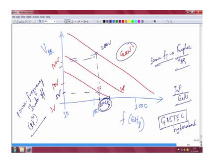
And what you can do is that you can plot the breakdown voltage on the y axis, on the x axis I can plot the frequency. So, suppose this is 10 gigahertz this is in gigahertz and suppose this is 100 gigahertz this is 1000 gigahertz 1 terahertz there is no transistor that will probably give a gain at 1 terahertz almost; very very you know very few indium phosphide is too close to 1 terahertz.
