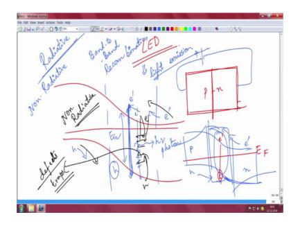
So, we will talk about LED; LED is the opposite of your photodetectors. So, what happens if that LED has to be a p-n junction ok. If you look at the white board here so, you have a p-n junction; this is p and this is n for example ok. The idea is that LED is also a p-n junction, a solar cell a photo detector can also be a p-n junction.
