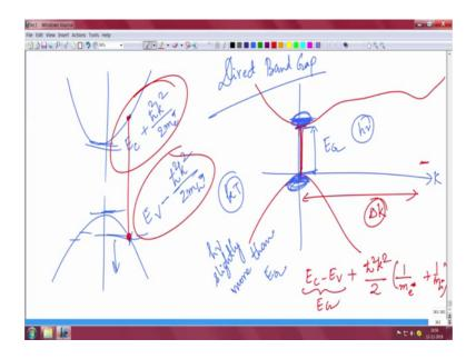
An LED can be made only from a direct band gap material that you know now right. So, it what it means is that in an E K diagram, if you have your conduction if you have your valence band like that a conduction band minima also should be on the same K.
