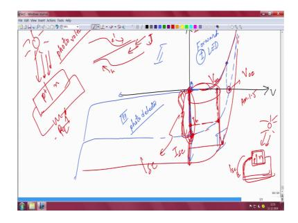
So, please remember that you are having an open circuit voltage when you are not keeping the circuit close; [FL] the circuit is open. So, this is the voltage that you are measuring across the p-n junction when you are shining light. If you short them no load is there then your current will be this at 0 voltage you are getting this much current, this is the quantity which is called the short circuit current.
