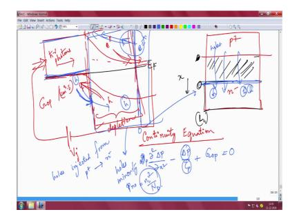
So, this is a solar cell and you know the recall the continuity equation, so I will take a probably simple case I will take a one sided junction which is a p plus and then n minus. Because it is p plus your depletion to the p side will be almost negligible, all the depletion will be on the n side only. So, this is a depletion region, ok.
