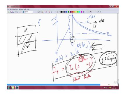
So, essentially based on this decay that is happening you can write down the diode equation, you have to solve this equation now. You have to in an idol diode equation you only this two terms, but now you also have an optical generation term. So, how you will solve with this equation and what do you will get as the solution; the solution will be say the current that is flowing.
