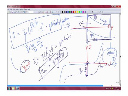
So, let us concentrate on this single junction only I mean the p plus n junction. So, in a way you are able to get the short circuit current of q the magnitude is q A Gop L p. So, what does it mean? You will see that the efficiency and the power output from a solar cell is higher if your short circuit current is higher of course, right that make sense the short circuit current.
