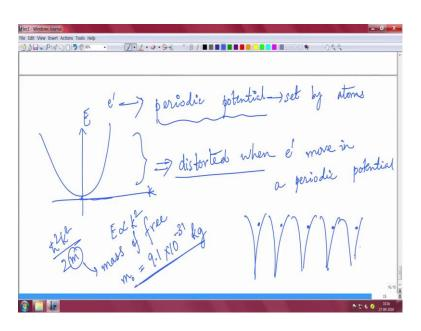
So, essentially an electron has to move in a periodic potential, it has to move in a periodic potential. And that periodic potential is set up by the atoms it right, all the atoms that are there in the crystal, setup this periodic potential and electrons have to move in the periodic crystal. So, when electrons move in a periodic potential in actually a semiconductor crystal like say silicon, then this E-k diagram that we have drawn know
