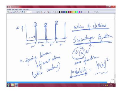
Remember a is the spacing between adjacent atoms, it is called lattice constant. Spacing between adjacent atoms ok, adjacent atoms, it's call lattice constant. It is also called lattice constant. So, so you have this infinitely deep potential well, this is infinity you can assume, this is infinite. And these are delta functions. You know where essentially you are electron, the nuclei of the atom slide, they are like delta functions, they are delta spikes and you have this periodic potential.
