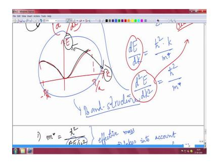
This E-k diagram that I told you that E-k diagram that I have been telling you here. This E-k diagram actually it is sort of a it is actually it is called a band structure this E-k diagram it iself is called band structure. How energy of electron changes its momentum that is actually call band structure. It comes from quantum mechanics. I told you it is very heavy physics. But the entire band structure information is actually condensed and you know crisply put into this  $d^2E/dk^2$  expression.
