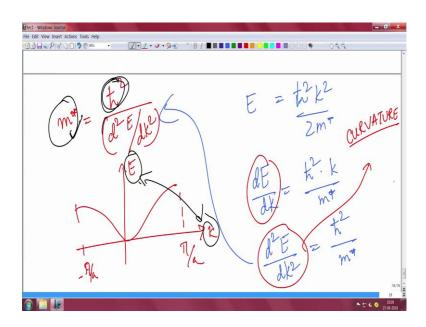
So, another way of looking at it is that if I write  $E = \hbar^2 k^2/2m$ , and then I take a derivative of E with respect to k ok, the slope of E-k diagram then I get  $\hbar^2 k/m^*$  right that is the derivative. Now, we take another derivative  $d^2E/d k^2$ , what do you get, you get  $\hbar^2/m^*$  square by m star.
