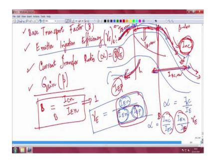
So, I will again draw the band diagram here. So, this is base emitter forward bias, this is base collector reverse bias, electrons that are injected here, some of them recombine, some of them reach here maximum reach here, once they reach here they are swept away here and collected here the holes also injected back injected which is a useless current component  $I_{Ep}$ , this components is  $I_{En}$  and the collector current here you get is  $I_{nc}$ .
