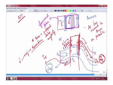
The way you operate a BJT the most common way to operate the BJTs so that you can get gain and other things is that your emitter and base this junction is forward biased. So, you will apply this is n, this is p, this is n, so you remember that this is a hole doping this is n. So, you forward bias the p this emitter base junction, it is a p-n junction that is a forward biasing.
