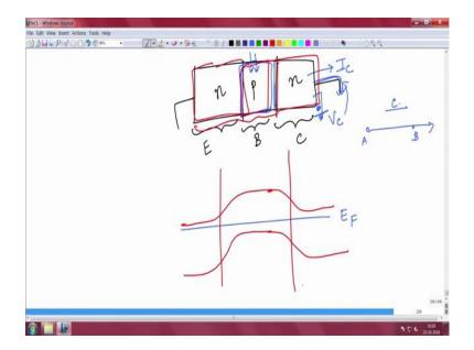
So, what did we tell in the last class I told you that a BJT is a transistor, it has two back to back p n junction diodes. So, I have an n p and then I have a p n I told you this is called emitter, this is called base and this is called collector. So, collector is typically the output where you collect the current and the current between and the current that is coming out at the collector is actually dependent on the input at the base, so that is how you control the current.
