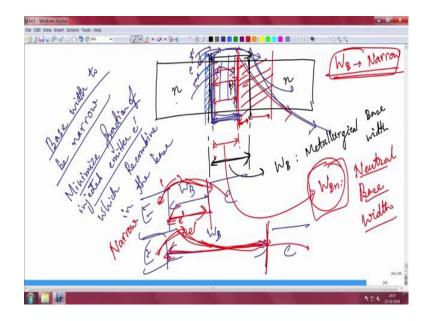
Now if you again look at the band diagram I will draw the structure again. So, this is suppose your let me draw a bigger structure so that I can correlate easily. So, this is your the schematic. So, suppose this is emitter n type, this is base p type, this is emitter again, this is collector.
