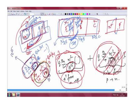
And this is emitter, this is base, this is collector each of this is n, this is p, this is n, you will have different doping this is n type doping, this is p type doping, this is n type doping, but the n type doping and emitter and collector could be different and the  $N_D N_D$  is not a good way.
