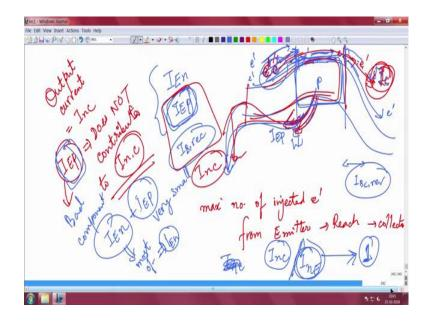
So, let us draw the band diagram again under operation. So, based emitter is forward bias and the base collector is reverse biased ok. So, electrons are injected from here there is some of them recombine they fall here and as soon as they go to the edge they immediately swept away here ok. So, I told you there is a base collector reverse bias here  $I_{BC,rev}$  which we typically ignore.
