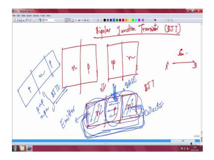
And we will see how a BJT is a Bipolar Junction Transistor the word popular says that both electrons and holes will be there, it is a Bipolar Junction Transistor it's call BJT and this is one kind of transistors which essentially changes the profile of the carriers. So, that you know you can tune how many carriers actually go down how many do not go and that way you control the current between two points A and B, A and B is controlled by the third point C.
