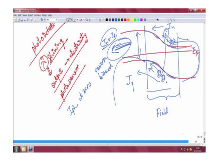
So, if we have the Fermi level and then you have this p n junction here, you are shining light suppose in this region, the depletion region there is a field here you know that there is a field here because the I have been telling you that many times that there is a slope in the conduction band.
