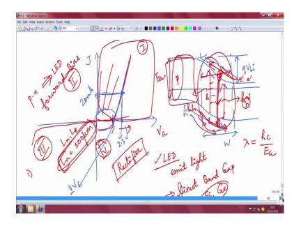
So, if you recall a p n junction in equilibrium you know has it's own depletion length depletion width you can say W and as I told you that if you apply forward or reverse bias, the depletion width can either increase or decrease. The built-in potential that you have here the voltage that you have dropping here, the built-in potential can also increase or decrease depending on whether you are applying forward or reverse bias right.
