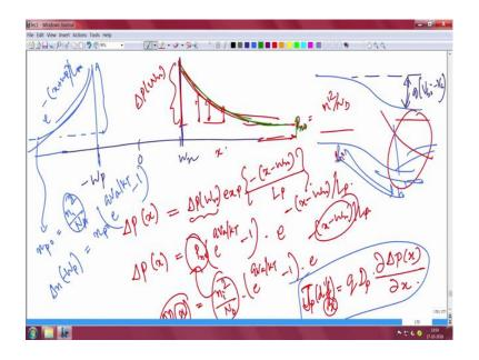
In the solution of the forward bias when we are discussing the forward bias condition here. There is a boundary condition that you know at large distance eventually your carrier concentration will become equal to the background carrier concentration right at large distances. So, that is one of the conditions for in this case when you have a minority in reverse bias junction.
