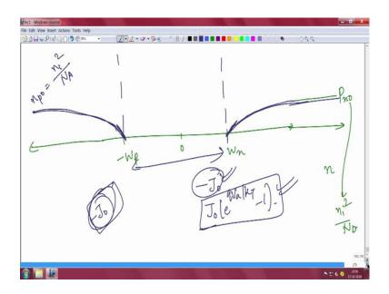
For example here so what is the condition that will apply, so essentially here I am drawing x this is 0 this is  $W_n$  this is minus  $W_p$ , the total carrier concentration at the
