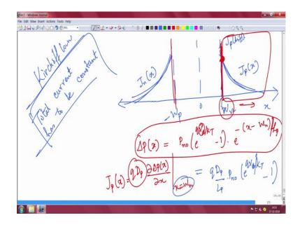
So, the hole current and the electron diffusion current will decay on the other side, if you recall the so I will talk about say only the n side how the holes are decaying because, the same thing can be applied to the p side. So, I told you the excess holes on this side will decay as  $p_{n0}$  which is  $n_i^2/N_d$  ( $e^{qVa/kT}$ -1)  $e^{(-x-Wn)/Lp}$  that is the applied voltage V a is the applied voltage the holes will diffuse.
