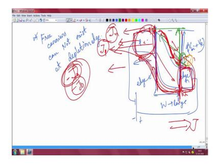
So, I will draw a reverse bias junction a reverse bias junction the depletion becomes larger. So, this built in voltage has become large by  $q(V_{bi}+V_R)$  it is a large which has increased now, because this is p type connected to negative this is n type connected to positive carriers are being drawn away. So, of the depletion region the depletion region has also become large in reverse bias what is happening is that holes are not injected and this side right.
