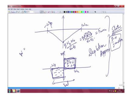
And I told you that your field electric field if you recall this is W n this is minus W p the field actually is maximum here and goes like that this maximum field is remember q N D W n /  $\in 0 \in S$  which is also equal to q N A W p / $\in 0 \in S$ .
