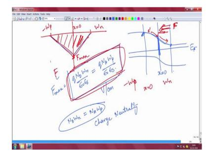
But, because field is negative x direction the field will you know essentially look this is x equal to 0. And plotting the field here is x equal to W n this x equal to now as W p. This is the maximum field and field will look actually like this I mean instead of positive it is basically negative everything else is same the value and everything is same. The field is actually in the negative side.
