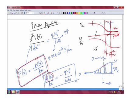
This is the Fermi level for example, this is the conduction band, this is the valence band. I am talking only of this part right only of 0 to W n at the end of W n here the field becomes flat after that there is no field; which means at x equal to W n. Your field vanishes because the field exists only here.
