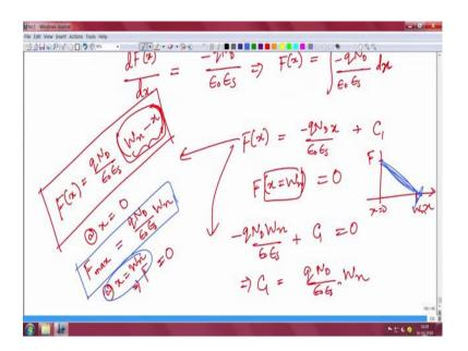
So, the first boundary condition is that F at x equal to W n will become 0. So, in this I will put F equal W n. So, it will become (-q N D W n )/  $\epsilon_0 \epsilon_s$  plus C1 is equal to 0
