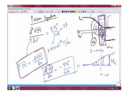
So, if I focus on that then I will draw it in a smaller scale. So, that we can good analysis also do the mathematics at the same time. So, this is the thing ok. So, I told you that this is your say junction x equal to 0. We are going to concentrate on this part which is x equal to 0 to x equal to W n. So, this is the depletion on the n side, the field exists in this region also the field exists in this region also until this region, but we will consider only this region the field exists here.
