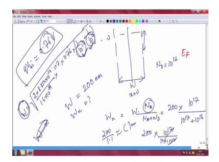
Divided by q which is  $1.6x \ 10^{-19}$  column into your epsilon of silicon is 11.7 into built in voltage qVbi which is 0.76. This into 1 by doping 1 by  $10^{17}$  by 1 by  $10^{16}$ ; so, if you do this you will find out the value of W. And it can be few 100 nanometer it depends on whatever right.
