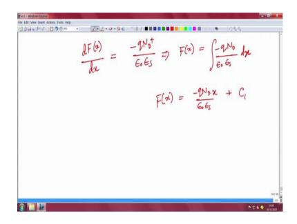
So, now we have to solve this equation dF/dx is equal to as q N D<sup>+</sup> / $\in_0 \in_S$  which means F(x) is equal to -q N D<sup>+</sup>. I can write this is -q N D only because N D<sup>+</sup> and N D are same. There is 100 percent ionization you know  $\in 0 \in S$  epsilon S into dx right into dx. So, I can see the field here. So, how will I do that now?
