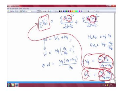
So, I will write it as qV bi is equal to q N D W n square by  $2 \notin 0 \notin S$  plus q and N A W p square by  $2 \notin 0 \notin S$ . Now you also recall that W is equal to W n plus W p because there is a total depletion with you also recall that W n times N D will be equal to W p times N A that you know the areal density on both side the same here.
