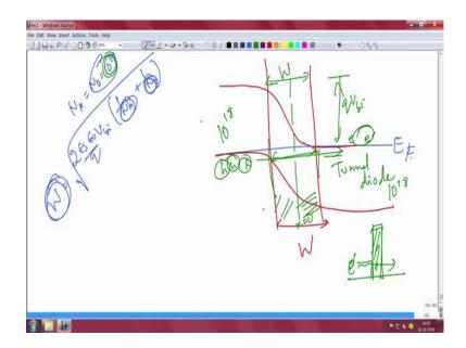
So, what will happen is that if this is your Fermi level. Then you are conduction band valence it will be very sharp depletion like this. It will have a very sharp depletion like the depletion; this is the depletion the total depletion is this. The total depletion is this is your x equal to 0 because the doping on both side is same  $10^{18} \, 10^{18}$  it will be the same doping on both same depletion on both side.
