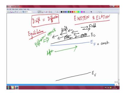
Einstein relation see Einstein not only had worked on relativity and gravity, but also there is a very important relation of Einstein in your semiconductor devices ok. So, suppose I take a sort of a material where both drift and diffusion current are basically going to balance each other.
