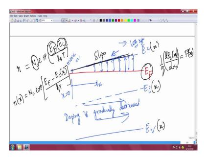
So, I have the Fermi level here ok and I have the conduction band like that and the valence band like that, it is still an n type semiconductor by the way because Fermi level is above the mid gap you know the mid gap will be here.
