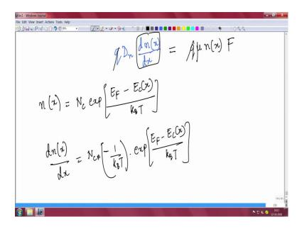
Now in this situation, I told you the net current is 0. So, the drift current has to be equal to diffusion current which means the diffusion current is  $q*D_n$ , because its electron dn/dx this n is a function of x why? Because if you look back into the previous diagram here at any point x here, sorry at any point x if I take this x is equal to 0 that at any point x here the electron concentration depends on x because this gap is increasing gradually right.
