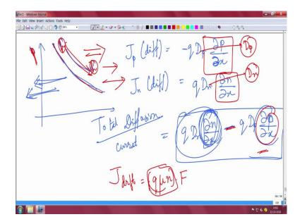
I told you that drift and diffusion equation depends on the slope of the carrier profile rather diffusion equation right. The electron and hole diffusion and the drift current does not depend on that you if you remember drift current you know was purely field dependent. So, that is for electron it is  $q^*\mu$  and which is conductivity times the field ok. So,  $\mu$  is mobility right.
