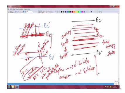
So, for example, I draw the band gap conduction band valence band I am not drawing the Fermi level here, but just conduction band valance band. Ideally this part should be forbidden gap there should not be anything here. It is clean band gap you know it forbidden gap.
