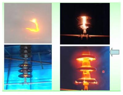
So various experiments with stand he flash over of single disk three disk were conducted.
