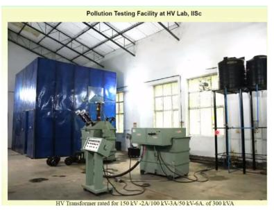
So for this facility was developed for testing the source and the pollution where in the source limitation we have is the 150 KV the current rate in is 6 amps where we can use up to 160 KV system so we tried to conduct the experiment on single disk where few disk in a strength in the limitation of a setup.
