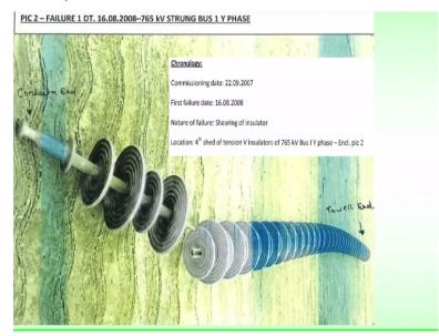
There are some failures even in the countries which are reported this could again would like to explain for the EHP insulators where the failures have happened at various junction you can see one of the failure is because of the brittle fractured happened after the fifth or fourth
