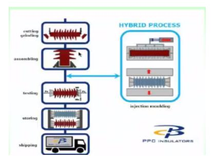
This figure shows the process of manufacturing for a regular post insulators and they the hybrid process here as earlier explained in the ceramic manufacturing ceramic insulator ceramic manufacturing we have discussed about the production aspects the manufacturing aspects of both the disk insulators as well as the post insulators here we briefly look into the process of comparison between the ceramic bushings or ceramic or post insulators mainly and the hybrid process which is involved.
