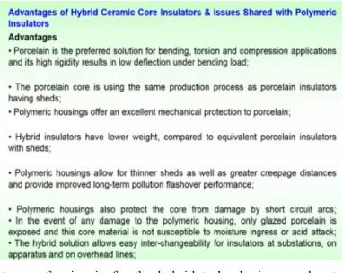
So there are advantages of going in for the hybrid technologies so advantages of this hybrid ceramic core insulators and some issues shared with the polymeric insulators have to be known. So if you are presented here so when you see the advantages porcelain is the prepared solutions
