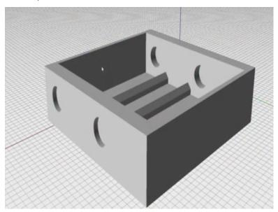
Basis for that design is the torch cell that is here. If you see here, any of these designs is based on a physical reality. Physical reality in this case is diameter, then what you call, the height, and then there is a small knob like thing at the bottom. This is where, what you call, a lot of reality check has to be done. Depending on the devices for which you are designing, you need to take the original.
