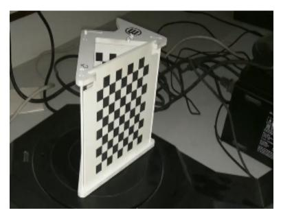
This is the device which is the scanner. And so you keep something probably I think this is the target which they have given and it is the maker bot target they have for the linearity and it rotates. And any object you can keep on it can be converted into a 3D file format and I will not say right now printing format is real otherwise it is a file.
