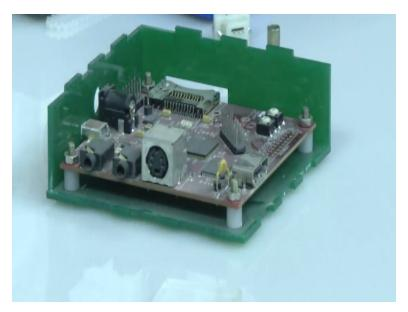
This is the one which I just showed you. In this case they have fixed this corner intentionally so that and then you see here I have a fastener that is fixed here and if I turn it over looks ugly, but does have a purpose and in this case, it prevents the surface from getting scratched when you keep it somewhere so you can even have decorative things. Now if I push it aside see this which I have shown you already.
