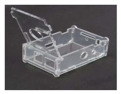
A hinge has been created. So even if you are to build these things in using a 3D printing techniques you can build these independently and this corner can be used that is you take this space, assemble these 2 together the hinge part is ready then after that try to assemble this and then once you put everything in place you have a hingable top cover.
