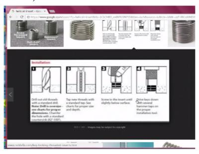
You have seen this know this is typically the way these helicoil stuff works. So you have a hole then you have a special what you call this thing here, then you have a device know which inserts the proper installation and so on. So this is standard practise when it comes to making this you know things in this. There is a good view about it here because often it is used more as a how to tell, is a repair but the reality is more than repair. It makes cents when we actually insert it like this.
