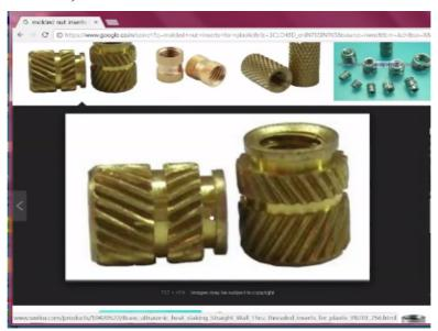
It looks a little like a gear wheel actually. Essential things what you need to notice is that a type of knurling like object has been created here. It is not actually a cross knurling, but then the advantage being about any of these things are it does not easily come out of the, it does not easily get ejected out of the what do you call the part. These are the most common thing which are used in normal injection moulded plastic.
