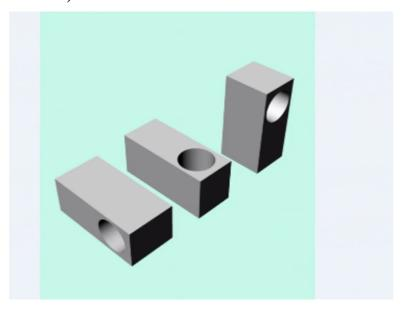
Now let us, we need to build this in our normal 3D printing machine. So if you are to make it such that this wire, this line, I mean the axis of this circular feature, cylindrical feature is normal to the surface meaning it is kept parallel, building here will be easy, absolutely no
