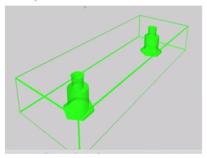
See this know, they are the edges of it and inside we have that small depression which approximates to the nutsert that I am going to push inside or the clinch nut which I am going to push inside and after putting the clinch in it I will have a surface you know which is again, I said 0.8 or 1 millimeter polycarbonate which is generally hard and depending on whether we have a what you call one adhesive which melts and sticks to that.
