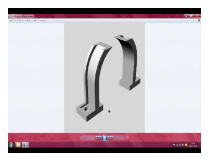
See here, what is happening? Now comes the other thing. After it crosses around 30 degrees, that overhang cannot be supported which is not possible to support the overhang. So lot of build material starting about here and up to here, up to here, up to here, same here, up to here, all this material gets wasted. But in some objects, we have no choice.
