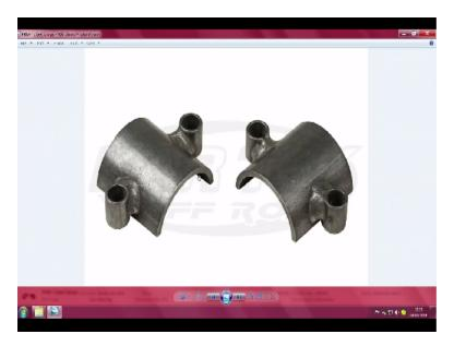
Imagine, this needs to be replaced using your 3M, I am sorry, not 3M, using your 3D printing object, now we have ended up with definitely a small issue. If you want to keep it flat like this and build with this way, this will require a lot of support and if you want to put it the other way, we still have a problem. This is where you need to take a proper decision. In spite of this, because of this long this thing and all that, I would rather build this in this direction.
