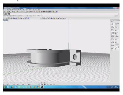
Now I need to take a call on what should be the counterbore which I make? Should the counterbore be done here or because of this thickness and to have the screw head to sit here, do you think I should extend this? Now you see filling it up, while it did make sense at one level, at one level, you will see that, you know, there is need to be a little compromise about it. That is the reason why probably this design was marginally better.
