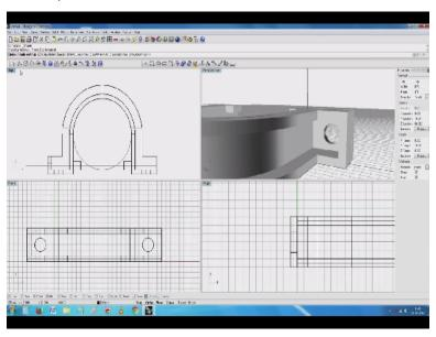
I will start with making a surface with corner to corner. See here, a small surface has been created and I will now extrude the surface. See here. What I wanted has now come without any problem, except that I know I did a goof up. So allow me to start again, try to make the surface again. This is slightly better, this thing. So this solid is going to be, see here. I have a neat box like structure.
