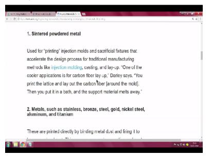
This is a very interesting thing, "used for printing injection molds and sacrificial fixtures that accelerate the design process for traditional manufacturing." You print the lattice and lay out the carbon fiber around the mold. Then you put it in a bath and the support material melts away. So you see here sintered powered metal is typically something which is used.
