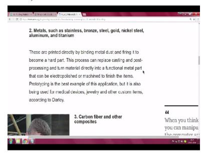
Next comes stainless rail, bronze, steel, gold, nickel steel, aluminium and titanium. Print it directly by binding metal dust and firing it to become a hard part. Process can replace casting and postprocessing and turn material directly into functional metal part that can be electropolished or machined to finish the items. Prototyping is the best example of this application, but also being used for medical devices, jewellery and custom items. So that you know, next lecture will contain.
