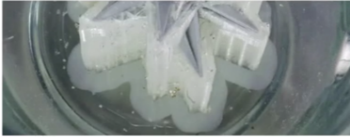
A print made with ABS print material and PVA supports with the Ultimaker 3
