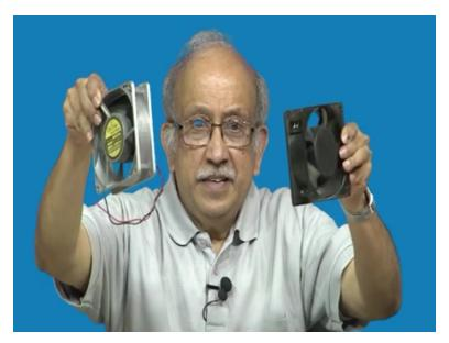
Imagine, now look at this. This is the fan I have been showing you all along. This is heavy. The part of it is made with a type of aluminum and there are 2 materials and you see the thickness. The thickness also varies depending on the power, the diameter and various things, I can change the material, as I want. There is a mild difference between the two and if you see next is, you see the way the blades are formed, can you see?
