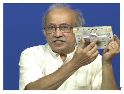
So after having searched everywhere we got this thing. This one is a heater which is built into flat mosquito pads. So at the bottom we have a heater and the whole thing has been what you call put together typically the rating of this is about 5 watts to 7 watts. So we did an experiment on this saying it is 5 to 7 watts is it okay. And then this one is taken from a insulin
