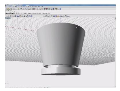
This forms a thermal bridge. See there I have a small plate which goes through this plastic and 1 or 2 features you will notice is it is not touching it anywhere. So that the heat is not directly affecting the plastic. I have left a small gap. Here I would like to give show your notice to any insulation all insulation works on the basis of trapped air. So if I make sufficient cautions such that the plate does not automatically touch the walls there is enough of an insulation.
