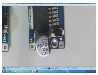
See this small detail here. So I need to support a hole here and I do not have much place here very little place is available for me same thing on this side also. If I come close you notice that this surface mount device capacitor is the limitation the amount of space has surface mount limitations. Similarly, here I have a small SMD another tiny I do not know probably it is a resistor and within this is where I have to support this hole.
