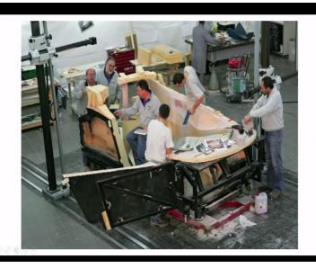
And then you see here, they have tried to make a door and then inside the whole thing is filled with polyurethane rigid foam structures inside and the later on they will cut it and you see here we have something else here on the top here. I am not very sure to be what it is, it could be a digital sculpting device or it could be what you call coordinate checking machine and so on.
