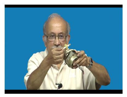
See here, this gear meets with this, got. Now you see here already, there is a reduction. Generally, there is a reduction may be of the order of 1:10 and so on depending on the pitch. While the speed is reduced, in our case a little desired effect is the torque has improved. Torque has increased tremendously because a big fan know has to rotate. Then, the second resultant thing for that is speed is reduced, torque is increased.
