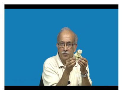
Now if you see the other side, one more small detail I wanted to show you. You see here they have given a small step here and left the remaining material, it is because in the case of injection molding it is very important that overall know total weight should be less and how the flow of material takes places very critically and runs all the drafts and all. In our case, if you see the other this thing, it may or may not be required like this.
