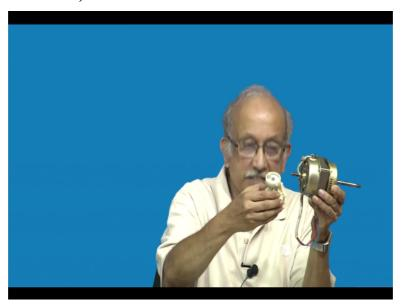
You see here, when I want to assemble it to this, when I need to assemble this mechanism to it, one of the first thing is it should have perfect alignment and randomly with the high speed when I try to push it now automatically alignment should take place. So there are 3 fixing screws, metallic again and then these are all bosses now here which will go and sit here like this. These are very, very convenient to do.
